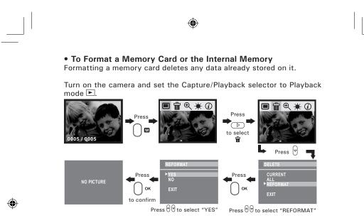
After the memory storage is formatted, the message "NO PICTURE" appears on the camera LCD screen.
